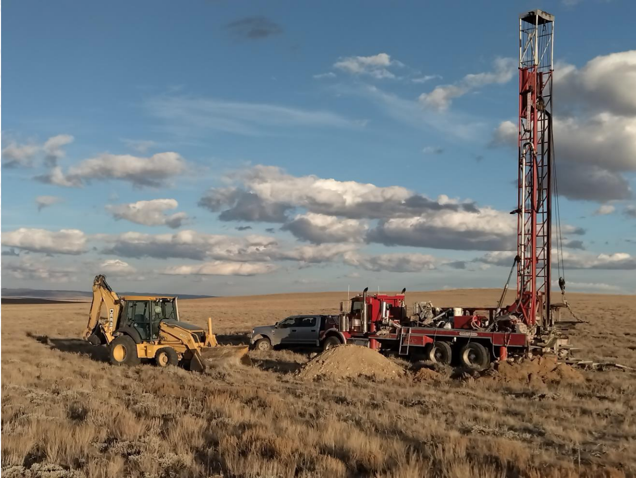
Mud Rotary Drill Rig Exploring for Roll Front Uranium Deposits
